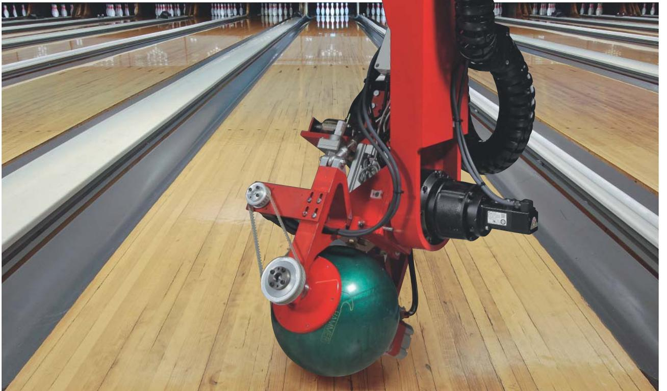
E.A.R.L. is able to release a bowling ball under test within 250  $\mu$ s of a scan of the position."
