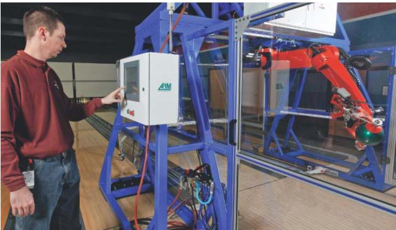
The USBC personnel can easily enter the test settings via a Beckhoff CP6901 Control Panel with a 12-inch touch screen display. There are 11 variables for configuring different throws to adjust speed and pick-up orientation. The E.A.R.L. robot can be reconfigured for completely different parameters in less than 10 seconds.
