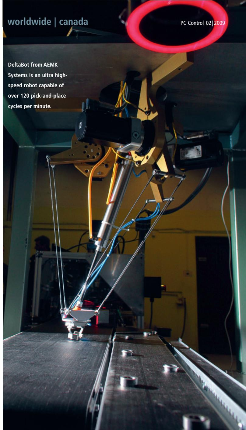
terminating factor in selecting the CX1010 as the DeltaBot's control centerpiece. We wanted the smallest possible footprint for the controller that would also give us the most programming flexibility," Khajepour said. "The basic DeltaBot configuration features the CX1010, however we can also easily scale up in performance using the CX1020 or CX1030 for the robots with an integrated vision option."
