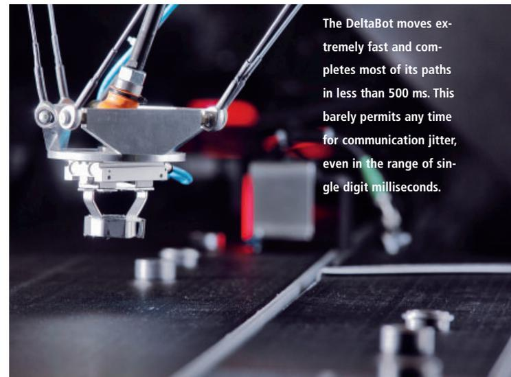
The DeltaBot moves extremely fast and completes most of its paths in less than 500 ms. This barely permits any time for communication jitter, even in the range of single digit milliseconds.
