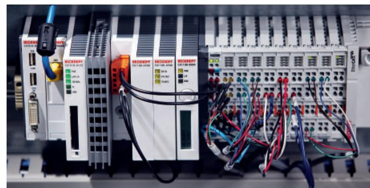
The DeltaBot line was recently upgraded with Beckhoff CX1010 Embedded PCs running TwinCAT PLC software to boost controls performance while reducing cost.
