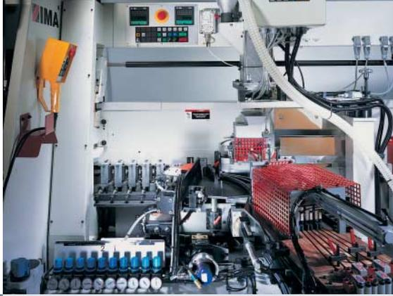
Gentle change-over: IMA implemented the change-over from “conventional” fieldbus technology to the real-time Ethernet solution in two stages. During the first phase, the Bus Couplers of the Bus Terminal stations were switched from Lightbus to EtherCAT. During the second phase the Bus Terminals were replaced with EtherCAT Terminals. Fieldbus slaves without EtherCAT interface can be integrated into the EtherCAT network via associated master terminals.
