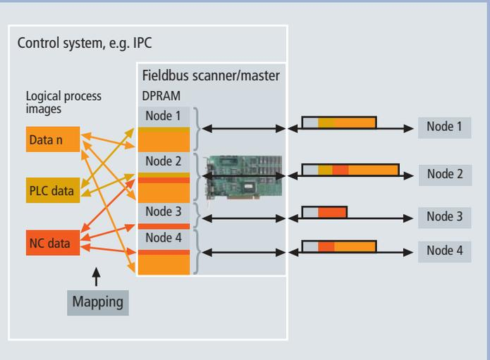
Conventional fieldbus systems generate a physical process image by collecting data of various types from the distributed nodes. The resorting (mapping) of the physical process image to provide a logical process image has to be done by the controller CPU.
