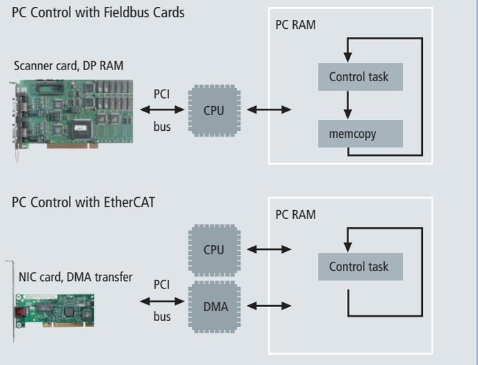
EtherCAT improves control system performance in a variety of ways. Besides the high speed network communication itself, the systems CPU is relieved by replacing the fairly slow byte-wise access to DPRAM of the fieldbus card by the Direct Memory Access (DMA) capabilities of the Ethernet Controller. Without CPU interaction data is made available in the main memory, which saves up to 30% processing power.
