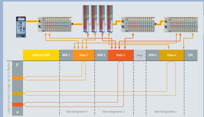
With EtherCAT, mapping is shifted into the fieldbus slaves and processed in hardware in the slave controller chips. The EtherCAT frame thus contains the logical process image directly. This takes further load off the master, since the resorting process is minimized.
