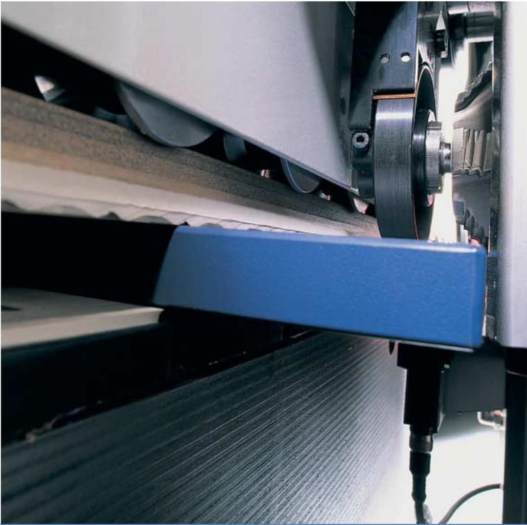
The Novimat Concept is a single-sided, automatic edge banding machine specially developed for jointing, edge banding and edge finishing while the material passes through the machine.
