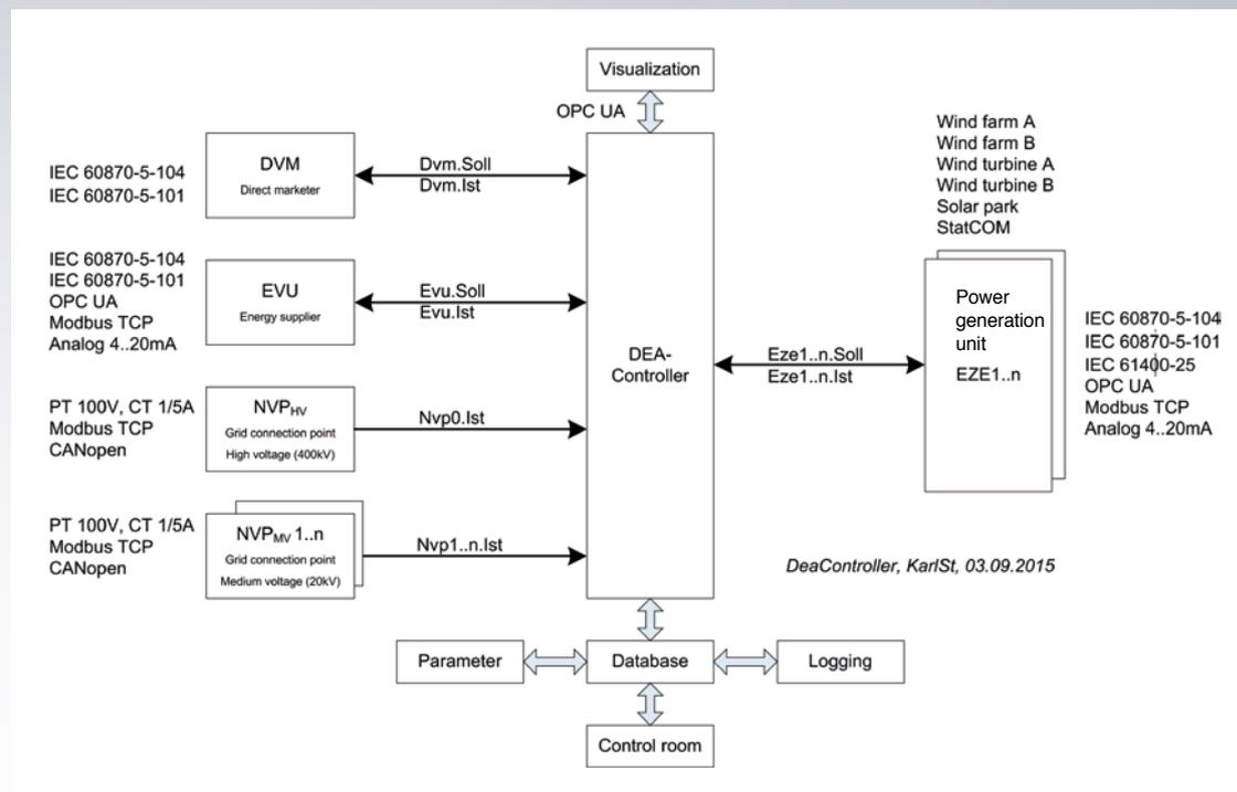
On the software side, each interface of the DEA controller is implemented as a modular function block with identical input and output interface. On the hardware side, various EtherCAT Terminals enable interface configurations that are optimized for the respective application.
