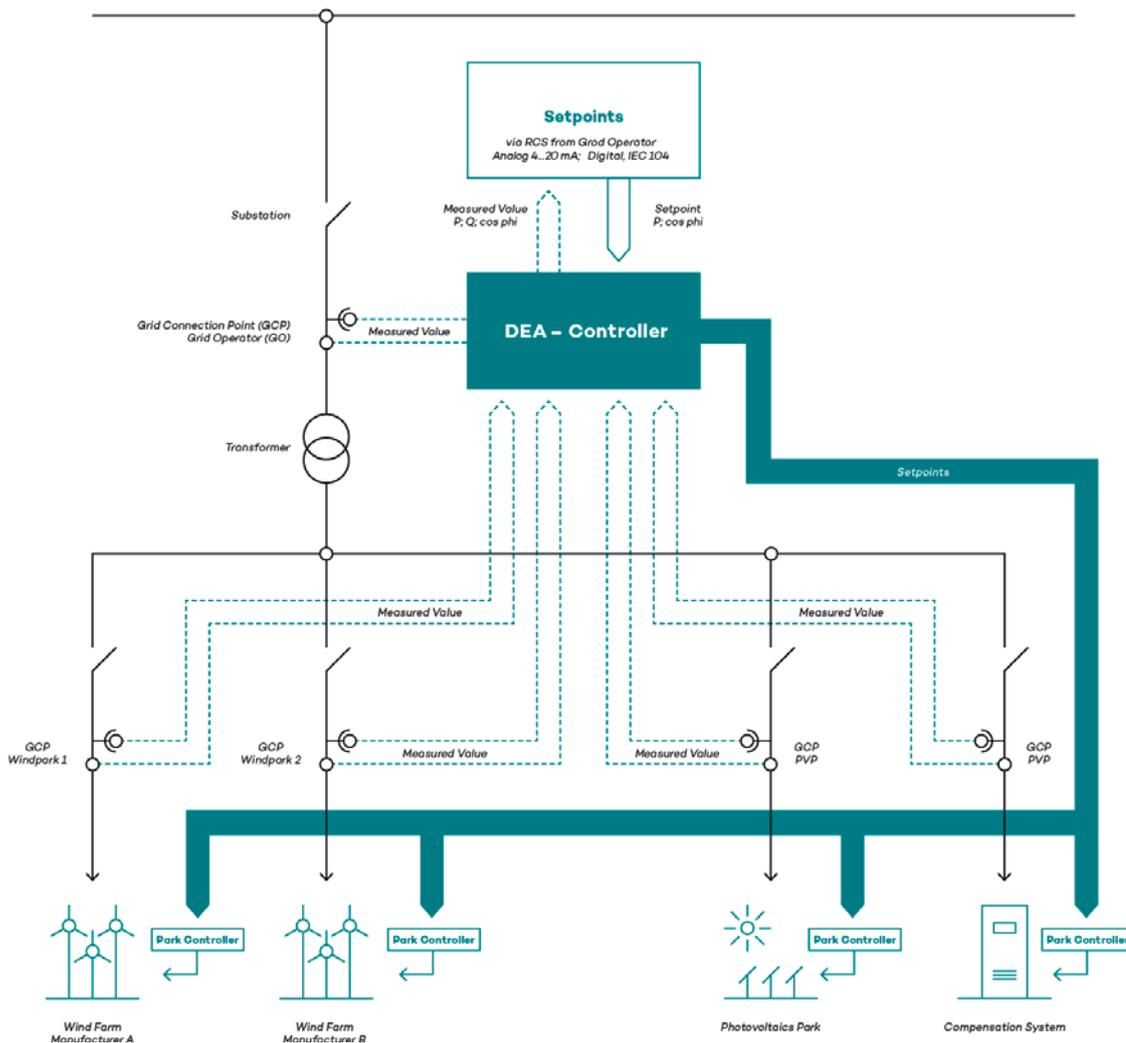
A DEA controller can be used wherever generating units from different system manufacturers share a common grid connection point, e.g. in situations with a shared medium-voltage transmission line or a substation for high-voltage connection.
