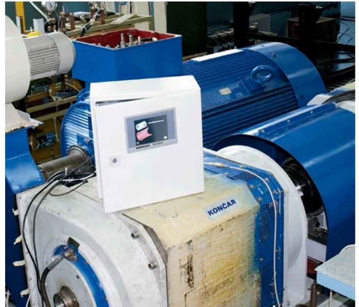
The EMCM developed by Končar is a comprehensive online condition monitoring system for low-voltage and high-voltage induction motors of any size.
