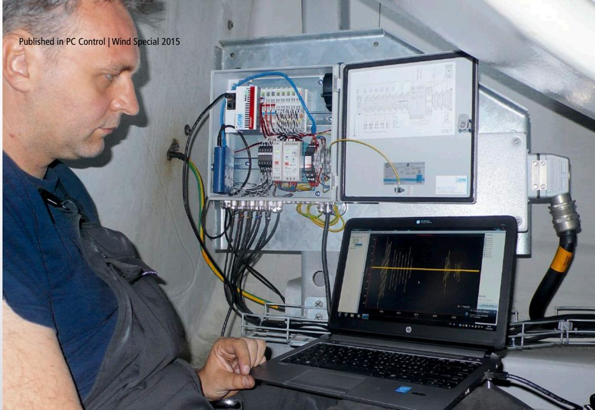
GfM staff engaged in testing acceleration sensors connected to the Peakalyzer.
