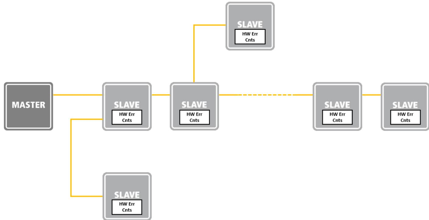
These memory addresses can be accessed by the master device and be provided to the control application (for example by means of dedicated variables, or via function blocks in the PLC program).
