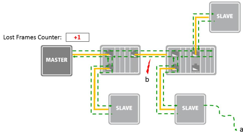
The master Lost Frame Counter can be considered as the first indicator of communication issues at hardware level in an EtherCAT network: an increment should trigger a deeper investigation by reading and interpreting [Hardware Error Counters](#) of slave devices.
