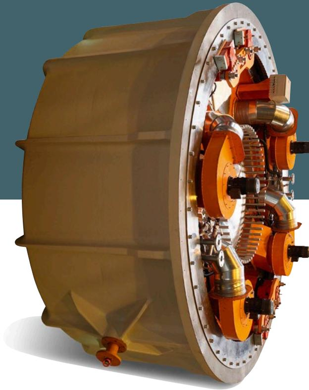
The permanent magnet generators (PMGs) from The Switch cover all wind power applications. Each PMG is designed with special magnet shapes and arrangements to match specific wind conditions for smooth operation and maximum efficiency. The directly driven, low-speed PMGs work without a gearbox, which results in an unequalled overall efficiency of the drive train.
