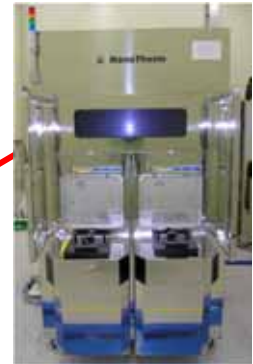
EFEM : End Front Equipment Module (Wafer Transfer System)
