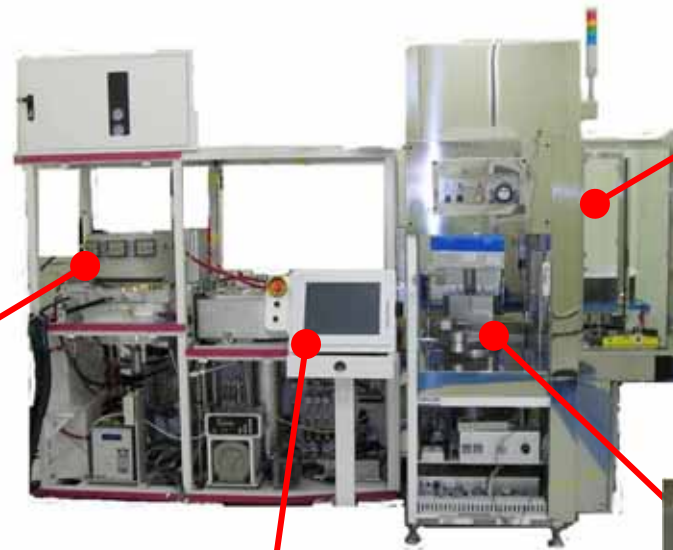
EFEM : End Front Equipment Module (Wafer Transfer System)
