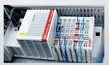
The condition monitoring system is supplied ready for operation, installed in a compact terminal box.
