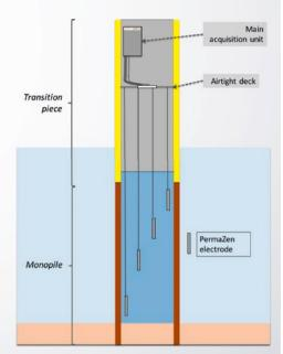
Electrodes are suspended at different heights in the water inside the wind turbine foundation. Between the electrodes and the wall of the foundation, voltage is generated according to a certain pattern. By comparing this pattern with the measured voltage and current values, a picture can be obtained of the corrosion activity on the surface.
