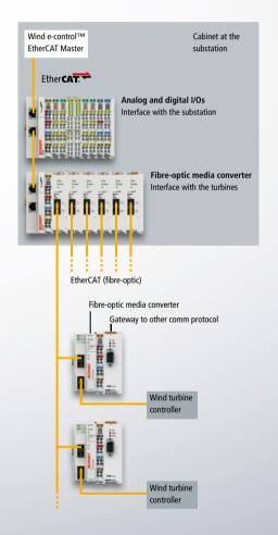
A general schematic diagram of the EtherCAT topology shows the functions handled by the individual modules in the wind farm.
