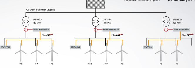
A Wind e-control<sup>™</sup> system is provided for each transformer station, securing the EtherCAT data transmission between the individual wind turbines in the wind farm.
