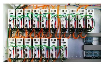
View of the central control cabinet of the Twins transfer system, on which small parts for gas fittings are manufactured. A total of fifteen 2-channel and two 1-channel AX5xxx EtherCAT Servo Drives are used for controlling the axes.
